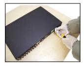
①disassemble the screw
