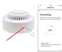
6. Press RESET for 5 seconds with PIN when configuration network, indicator flashes slowly, start manual network configuration mode. Input WiFi account and code to add device.
