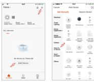
Press the RESET for more than 5 Seconds with the PIN, the LED indicator flashes quickly, start network configuration automatically. Input the WiFi code to start connecting.
